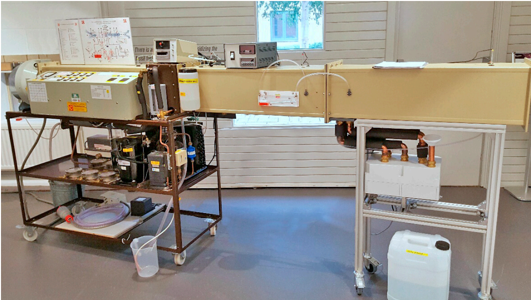
De Montfort - features additional bespoke evaporative cooling unit
